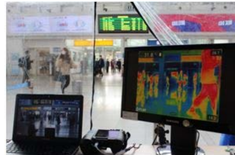
Thermal camera used by KORAIL in Korea
