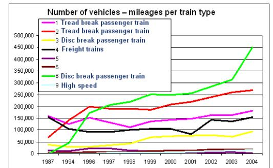
Still a considerable number of passenger trains with cast-iron blocks (type 1 and 2 ) is running on the Dutch network.
