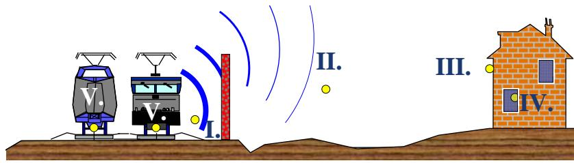
Figure 15: Positions where noise limits can be enforced.
