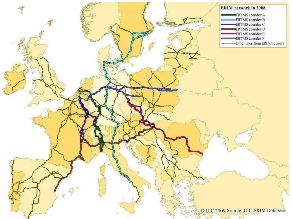
Figure 3: The rail freight oriented network and the main corridors (UIC Atlas 2008 of Infrastructure in the ERIM Network).
