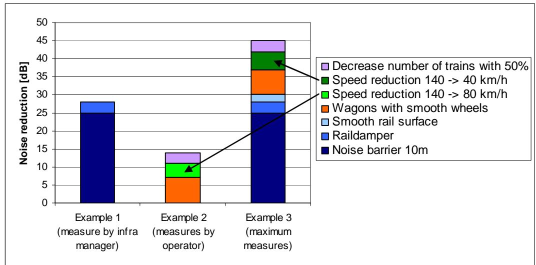
Figure 29: Effect of different noise measures on the reduction of railway noise.
