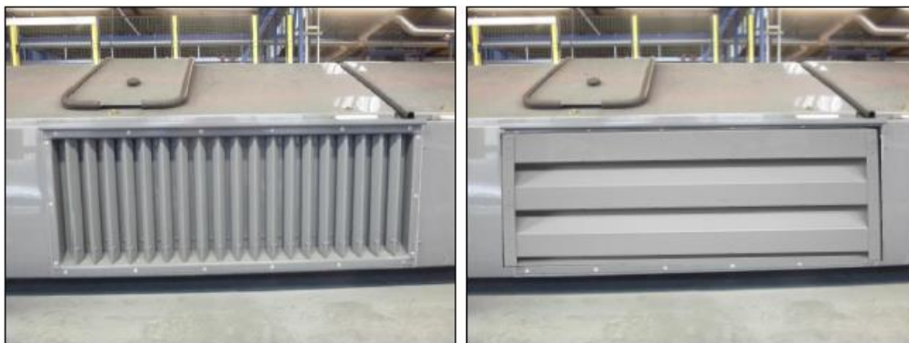
Figure 22: Fresh-air intake of a passenger HVAC (left: standard, right: acoustically optimised) [24]
