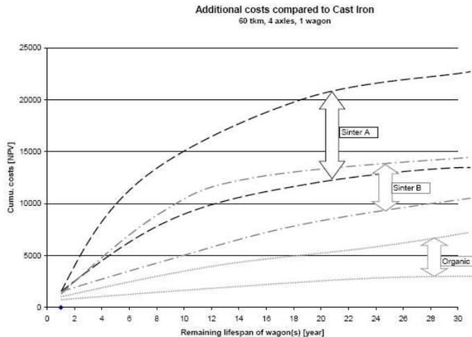
Figure: Influence of LL-blocks on LCC. [Source The Whispering Train Programme - Life Cycle Cost calculation – Intermediate Report – Lloyd’s Register]
