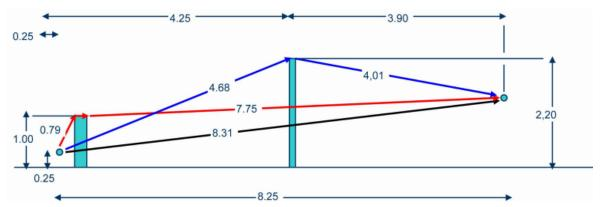
Figure 12: Geometric comparison of low height barrier close to rail with the usual configuration at about 4 m. The noise reduction is about the same in both situations.
