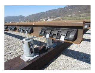
Photographs of the four main damper types. Pictures were taken during the car park tests in Hägendorf (see experience in Switzerland).
