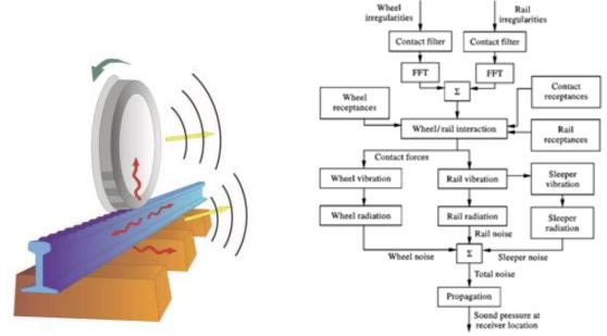
Figure 1 (left): Noise creation mechanism.
