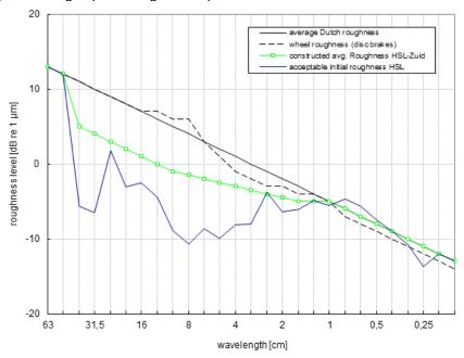
Figure 11: High speed roughness spectra
