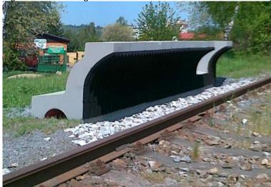
Also, prototype parts of rail noise absorber called BRENS ABSORBER were made in order to increase sound absorption of the rails. Laboratory measurements of noise attenuation were taken. Noise reduction achieved in the laboratory for the whole system was of 14 dB. Results for the barrier alone are not known.
